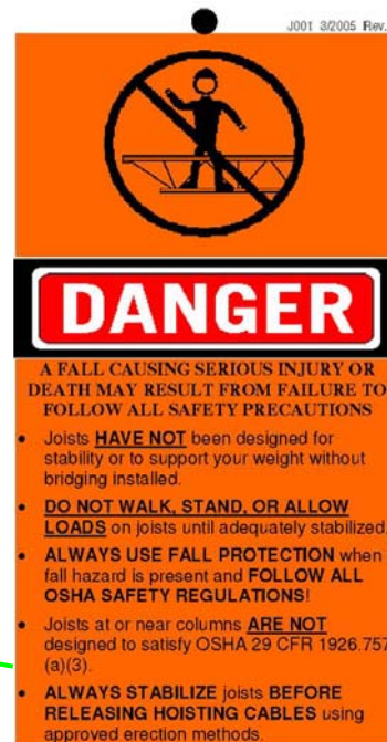
FIGURE 4 TYPICAL SJI MANUFACTURER’S DANGER TAG ATTACHED TO COLUMN JOIST
